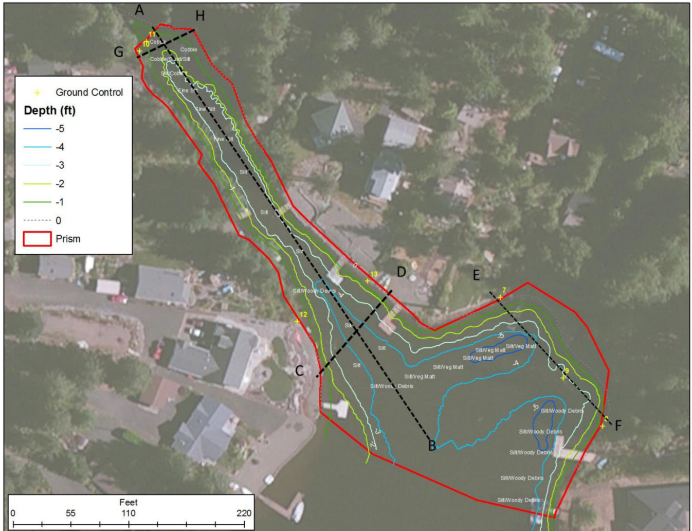
Figure 7-12 – Dredging transects in King's Cove
